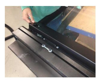
7.6. To replace the lock, loosen the two M6 Allen bolts that hold the locking mechanism in place.
