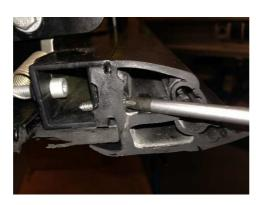
7.2. Pry the rubber foot out of the aluminium vertical profile from the bottom to the height of the lock cover plate.
