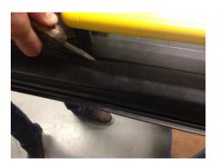
7.9. Put the screw back into its original place which secures the rubber to the vertical profile of the door leaf.
