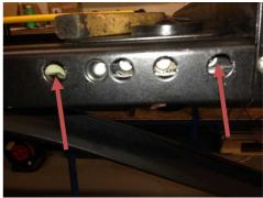
7.5. Remove the lock cover plate. Be carefully not to damage the paint which is easily damaged when removing the cover plate.
