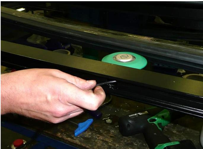
Remove rubber and pull out the cable of the EAO push button out of profile
