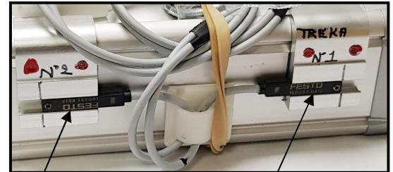
**Fig.1:1** Shows No.2 Reed-switch in the **WRONG POSITION**.
