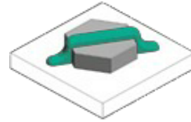
Figure 43: Mark the fasteners with a torque marker
