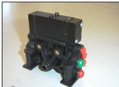
Example of side ported valve Follow same colour coding to cylinder(ram)
