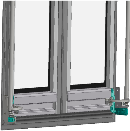
Figure 15: Catch wedge and catch block locations
