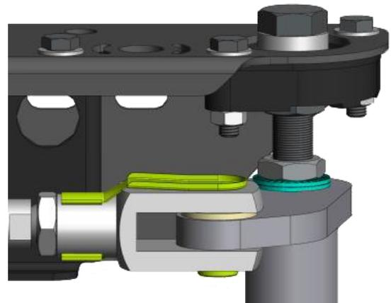
Figure 4: Secure nut with Nord-lock
