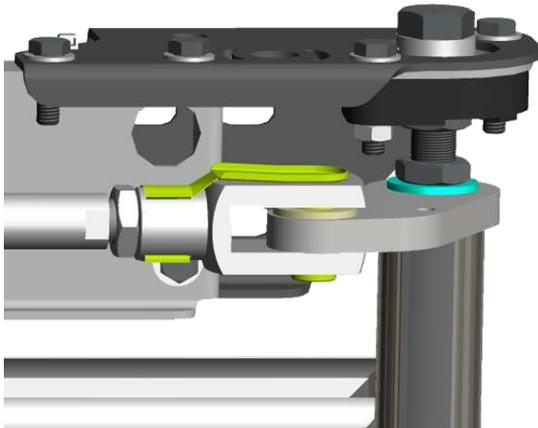
Figure 3: Secure nut without Nord-lock
