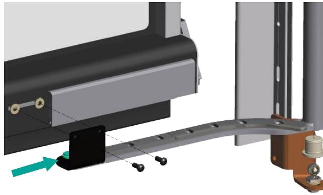
Figure 8: Lever bearing bush
