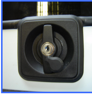
External Rotary Lock Handle. Key Can Be Removed In Open or Closed Position
