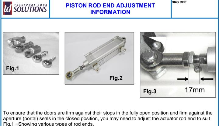
Fig.2 = Showing typical pneumatic cylinder facture pre-assembly
