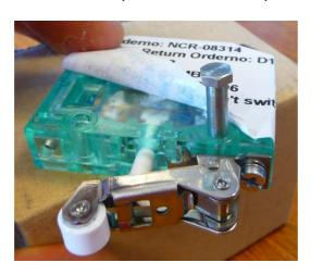
The picture below shows the shaft coming out of the mounting hole from underneath. This is important because the shafts prevents overtightening of the switch, which can cause a faulty switch.
