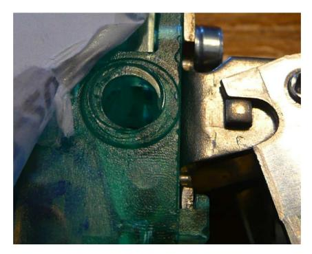
Damage like this is caused by using a fastener with a shaft that isn't long enough.
