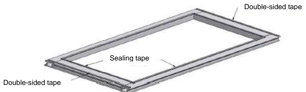
Figure 3: Applying sealant tape and double-sided tape to the door frame
