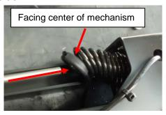
8.2.3. Tighten the bolts with a lock disc on both sides and fix the cable with a cable tie.
