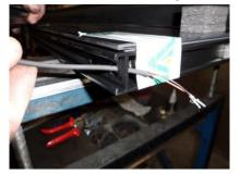
8.3.8. Glue the cable to this surface, then put the screw back in. The cable goes out through the profile.
