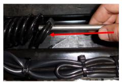
8.2.2. The rod goes through the hole on the side of the frame, so you can mount the cable on the other side.
