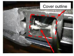
8.3.13. Slide the guiding bracket back, so that in open position the doors are perpendicular with the step edge. Tighten the bolts. The door
