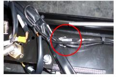
8.2.6. Remove the guiding shaft from the bracket (Topside of the door) and guide the cable on the bottom side of the mechanism through the shaft and the plastic cover. (Make sure the rubber ring is inserted in the cover!)
