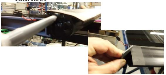
8.3.10. Put the pins of the sensitive edge in the connector as shown
