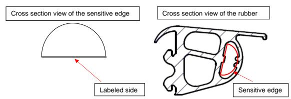
8.3.6. Insert the sensitive edge with the labeled side facing the door. On the bottom side of the rubber should be a clearance of 10-15 mm until the sensitive edge.
