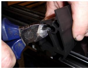
8.3.3. Remove the screw from the rubber.
