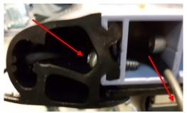
8.3.9. Seal the topside of the rubber to prevent water ingress. Remove the excess sealant
