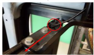
8.3.12. Connect the sensitive edge with the spiral cable and put the excess cable back in the profile. Be aware of the tip of the screw, as this can damage the cable or yourself! Put the plastic cover on the profile.
