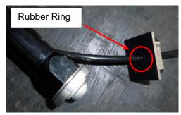
8.2.7. Insert the wires in the connector. Now the mechanism is ready to be connected with the door.
