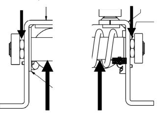
• After you have done this de bearing shafts will come off and you can remove the bearing from the shaft.
