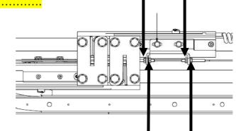
• First loosen the cable connecting the two bearings, using the tension nuts.
