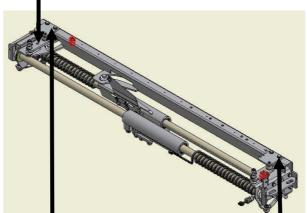
• Place the suspension plates back on the frame en tighten them make sure they are pulled back so the hinge is leveled.
