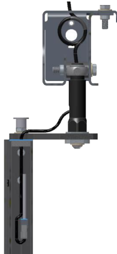
Figure 1: Spiral cable runs smooth and has no overlength
