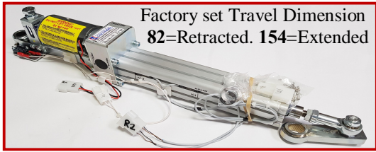
Fig.1:1 Shows No.2 Reed-switch in the WRONG POSITION .
