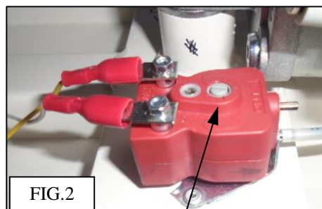
FIG.2 Adjusting screw Clockwise=heavy detection Anti-clockwise=light detection
