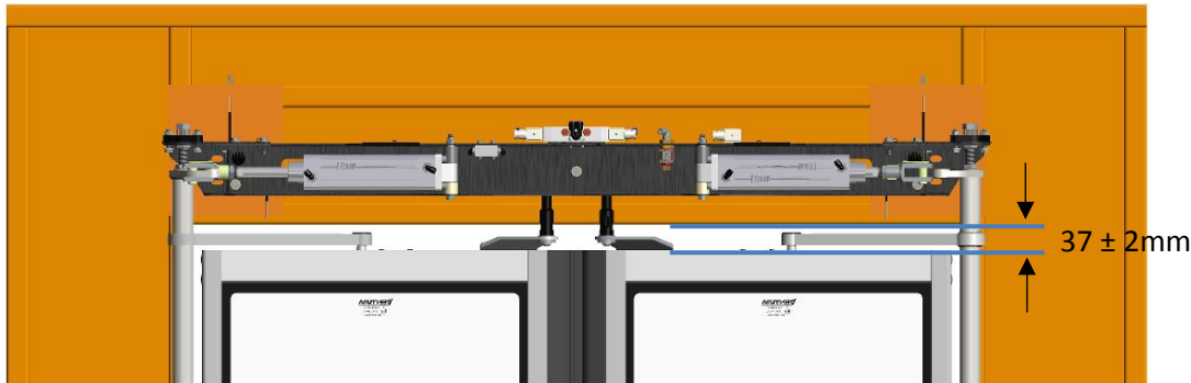
Figure 1.1: Check door height (distance between door leaf horizontal profile and aperture)
