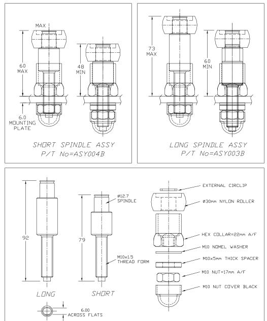
For typical doorguide spindle assy replacement installation sheet see INST-100-07.
