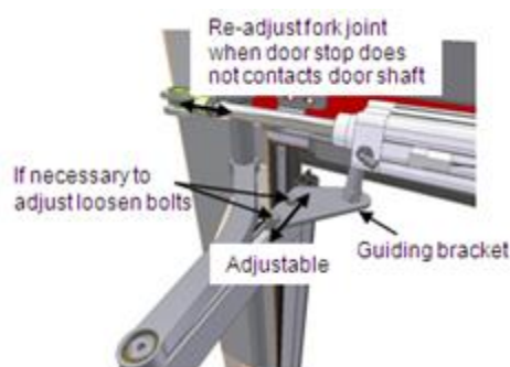
Figure 1.16: Adjusting guiding bracket
