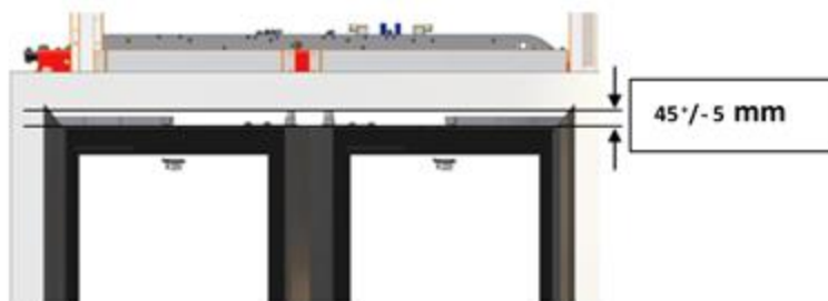
Figure 1.8: Check door height (distance between door leaf profile and aperture)
